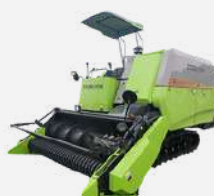
Crawler Self-Propelled Bailers
